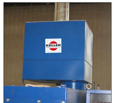
TRGS 560 requirements are met with the optional H13 secondary filter and clean air recirculation back into the room is possible.
