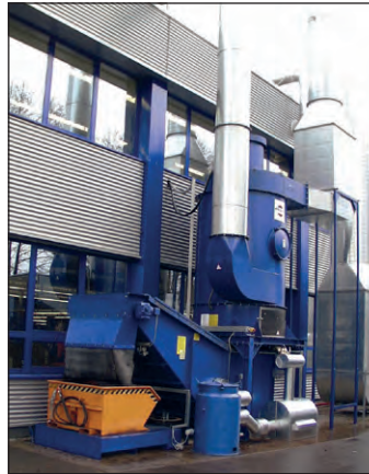
Wet scrubber VDN-AS with de-sludging device
