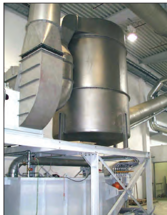
Wet scrubber VDN-TA in stainless steel design
