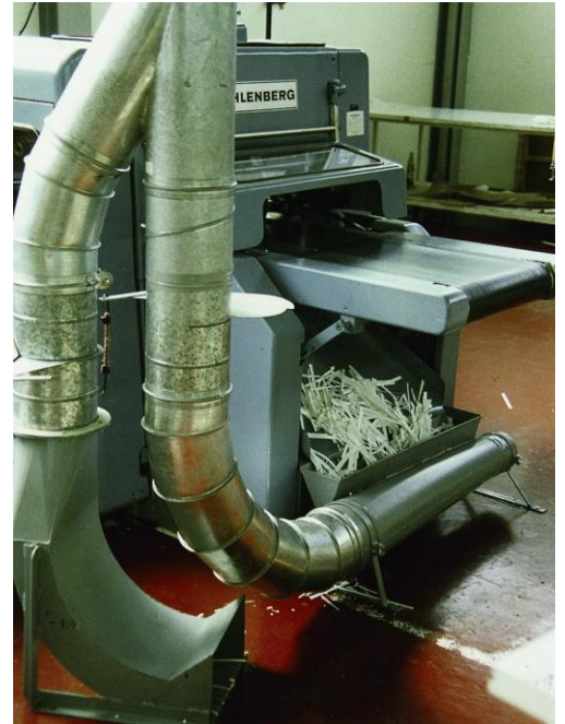
Collection element combined with chute
