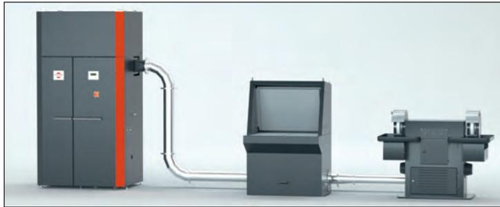
HydronPlus connected to a Keller downdraft table and brushing machine
