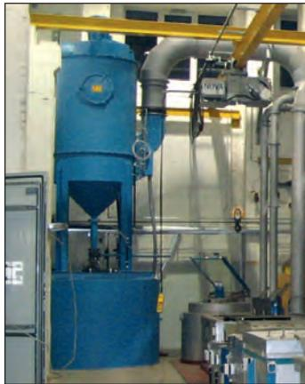
Wet scrubber VDN-T with water holding tank
