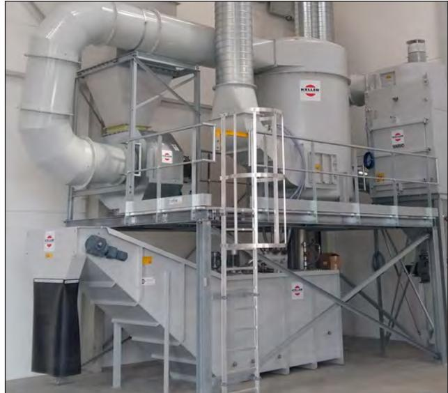
Wet scrubber VDN-TA with sludge remover
