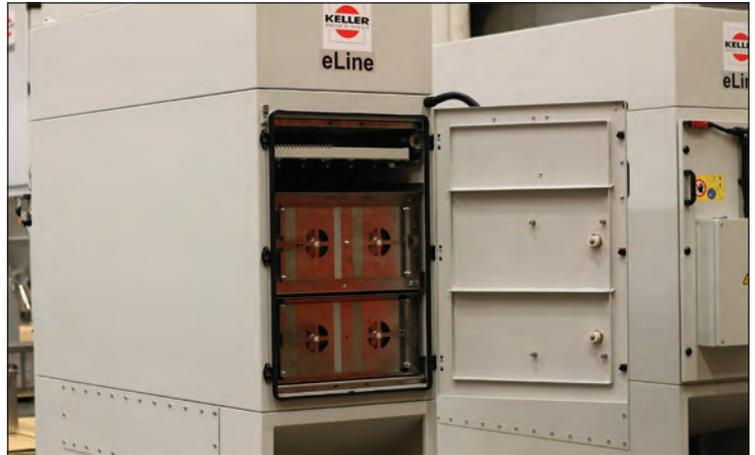
The separation principle is based on the fact that positively charged particles and similarly charged plates repel each other.
