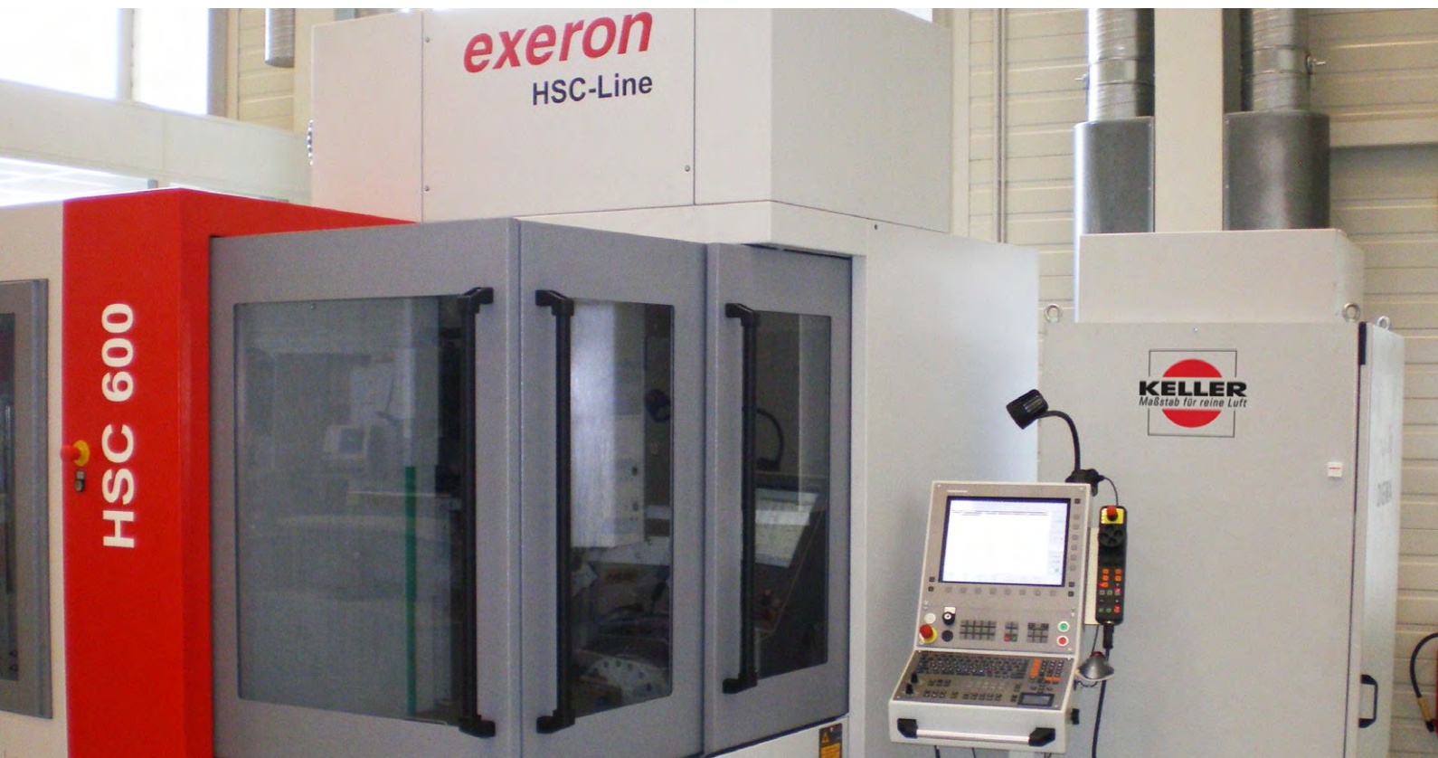
Extraction of a High-Speed-Cutting-Center with VARIO T 1.0 dry separator
