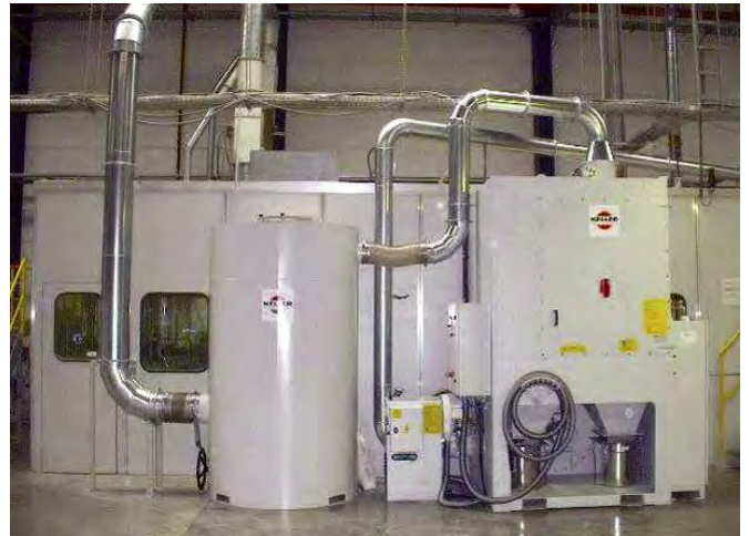
Example of a designed system, L-Cut 4 DOS with activated carbon filter automatic CO 2 extinguishing system
