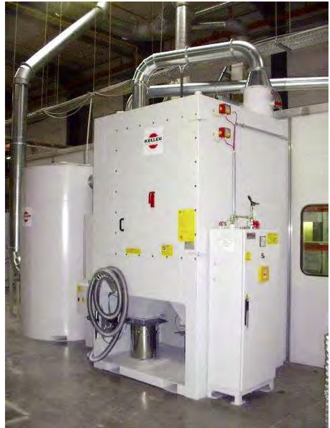
Laser processing of Example of a designed system, L-Cut 4 DOS with activated carbon filter and automatic CO 2 extinguishing system
