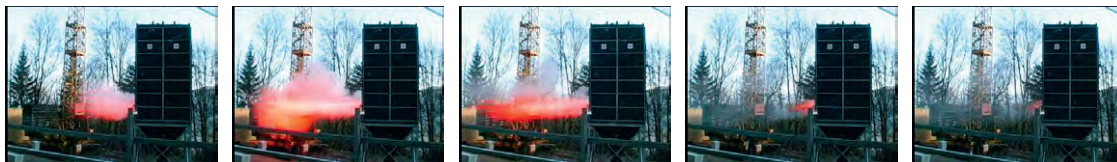
Testing the explosion potential of filter housing at the FSA facilities
