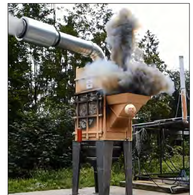
Explosion suppressed by ProPipePlus
