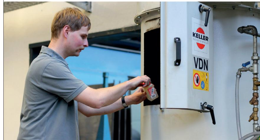
Tim Daffner, Synlab employee, tests the water properties in a wet separator
