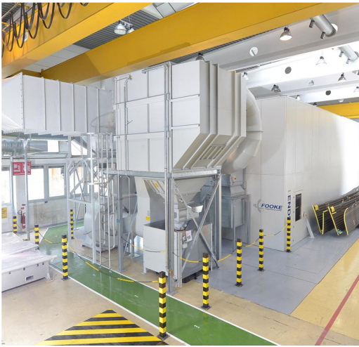
Image 1: The complete package consisting of Fooke milling machine with enclosure (in the background) and Keller Lufttechnik dust extraction system (in the foreground), exactly met the operator's requirements and considered all standards.
